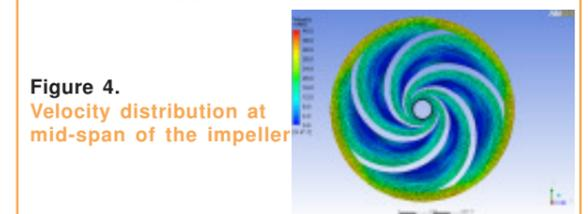
Figure 4. Velocity distribution at mid-span of the impeller
