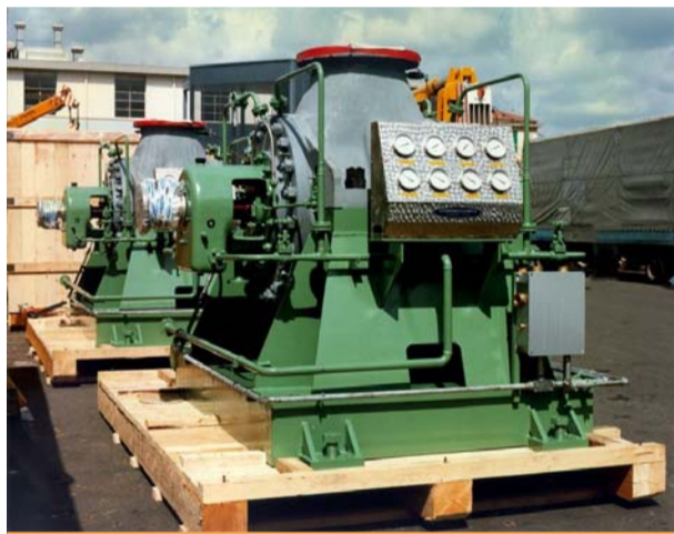
Cernavoda Nuclear Power Plant Booster Pumps - pump type 400 DP 80
