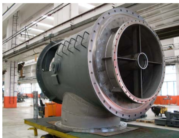
Discharge elbow made of mix of carbon steel and stainless steel, type 316L, to be installed in a Pakistan plant
