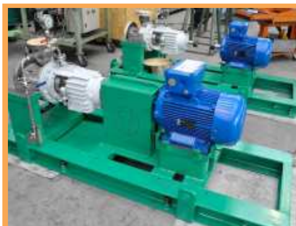
Horizontal overhung centrifugal pump single stage series AP type OH2
